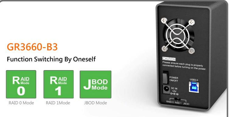
GR3660-B3 has three configuration modes built-in: RAID 1 (Safe Mode), RAID 0 (Speed Mode), and JBOD (Two Independent Volumes) for you to choose according to your needs.
